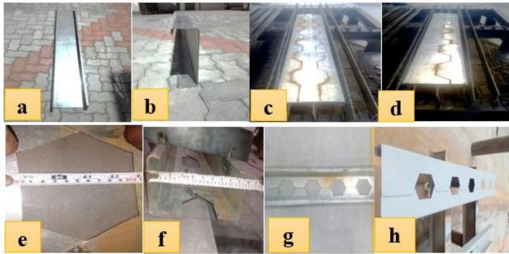
Figure 1 (a) C shaped - Cold formed steel section (b) Cross sectional view- C shaped - Coldformed steel section (c) Plasma torch cutting pattern -1 (d) Plasma torch cutting pattern -2 (e) Hexagonal dimension pattern verification (f) Overall dimension verification (g) Castellated beam-assembled section (h) Primer coated with finished coldformed metal surface.
